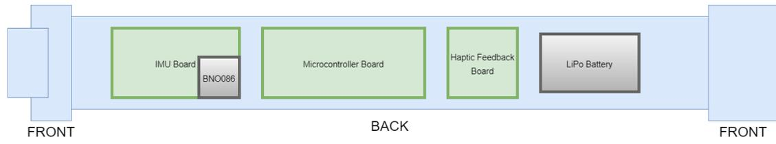
Figure 3: Physical Diagram
