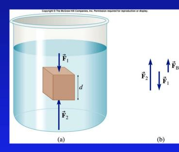
• Buoyant force is weight of displaced fluid!
