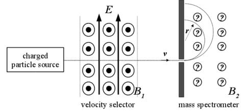
1. The velocity selector is set up to select positive charges only.
