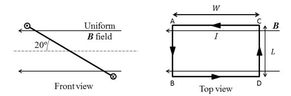
A rectangular loop of length L = 0.445 m and width W = 0.285 m carries a current I = 3.9 A is exposed to a uniform magnetic field of magnitude B = 5.5 T, as shown in the figure.
