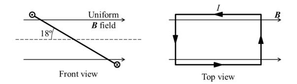
A rectangular loop of area  $A = 0.0245 \text{ m}^2$  and carrying a current I = 3.9 A is exposed to a uniform magnetic field of magnitude B = 4.6 T, as shown in the figure.
