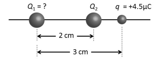
1) What must the value of  $Q_I$  be such that the force on q due to charges 1 and 2 is zero?
