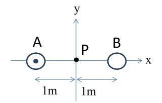
5. If the current through wire A is 1 A and no current flows through wire B, what is the magnitude of the magnetic field at point P?
