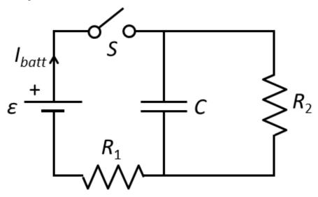
15) What is the current out of the battery, *I*<sub>batt</sub>, immediately after the switch is closed?
