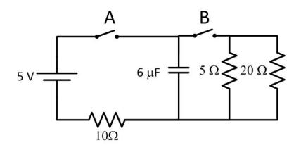
5. Switch A is closed at time t=0 and switch B is left open. Which graph shown below best represents how the voltage  $V_C$  across the capacitor changes with time t?
