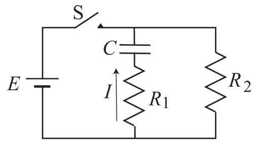
11) Switch S has been closed for a long time. What is the current *I* through  $R_1$  immediately after S is opened? Pay attention to the direction of the current arrow in the figure.
