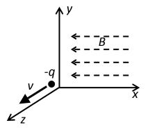
25. An electron (mass:  $m = 9.11 \times 10^{-31}$  kg, and charge:  $q = -1.60 \times 10^{-19}$  C) is initially at point  $P_1$  with speed  $v_1 = 3.1 \times 10^4$  m/s. It is moving in a uniform magnetic field of strength B = 0.15 T. How fast ( $v_2$ ) is the electron moving when it reaches point  $P_2$ , which is  $d_1 = 2.5 \times 10^{-7}$  m along B and  $d_2 = 1.5 \times 10^{-7}$  m perpendicular to B with respect to  $P_1$ ?
