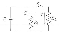
Initially, switch S is open for a long time. After t=0 switch S is closed. Choose the best figure from below describing the time-dependence of the current I through  $R_2$ . Do not forget that the battery E is still connected.
