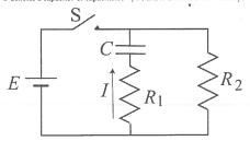
11) Switch S has been closed for a long time. What is the current I through  $R_I$  immediately after S is Switch S has been closed for a long time. What is the current / through  $R_1$  immediately after S is opened? Pay attention to the direction of the current arrow in the figure.
