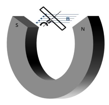
A coil of wire turns between the poles of a permanent magnet as shown in the diagram. The coil has N=34 turns of wire. The magnet produces a constant field of magnitude B=0.119~T. The coil has a cross-sectional area  $A=0.0411~m^2$ .
