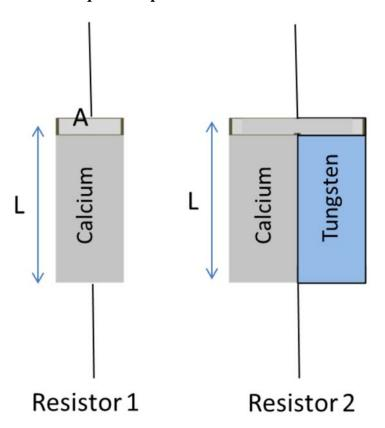
A student decides to build some resistors using rectangular blocks of calcium ( $\rho$  =3.36 × 10<sup>-8</sup>  $\Omega$  m) and tungsten ( $\rho$  =5.6 × 10<sup>-8</sup>  $\Omega$  m). The dimensions of the blocks are identical with a length L = 0.12 m, and cross section A = 2.25 × 10<sup>-4</sup> m<sup>2</sup>. Resistor 1 is created from a single block of calcium. Resistor 2 is created by attaching a block of calcium to a block of tungston as shown in the figure above.
