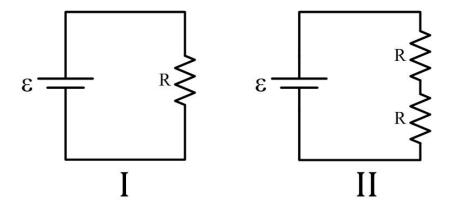
Which of the following statements is true regarding the power  $P_I$  supplied by the battery in circuit I compared with the power  $P_{II}$  supplied by the battery in circuit II?
