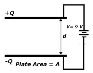
A parallel plate capacitor consists of two metal plates with an area  $A = 542 \text{ mm}^2$  separated by a distance d = 0.36 mm. The capacitor is connected to a 9 volt battery as shown above.
