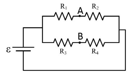
8. If all four resistors have resistance R, what is the total equivalent resistance for this circuit?
