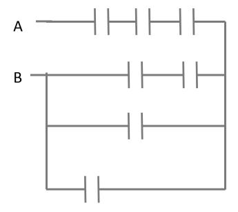
What is the equivalent capacitance of this network between points A and B?
