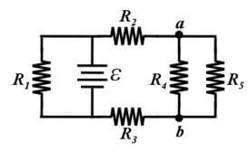
13. Assume all of the resistors have resistance R. What is the equivalent resistance,  $R_{eq}$ , for the circuit?
