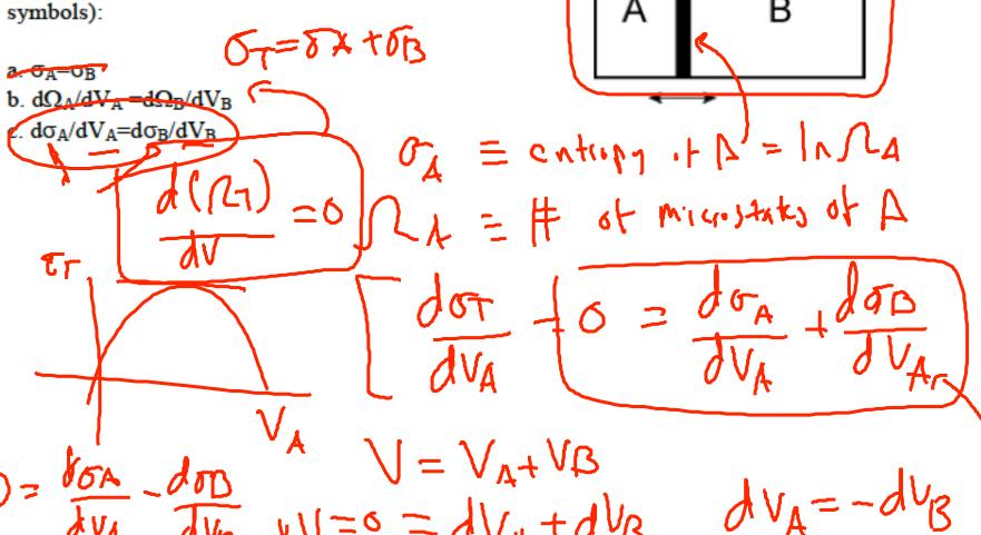
An isolated system in internal thermal equilibrium can be in either macrostate A with entropy  $\sigma_A = 27$  or macrostate B with entropy  $\sigma_B = 20$ . A particular microstate X is part of the A macrostate, and a particular microstate Y is part of the B macrostate.
