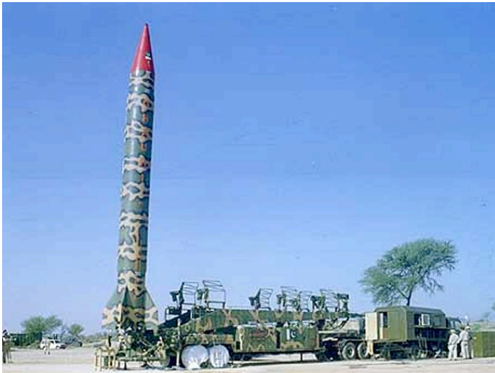
Pakistan's Ghauri MRBM and transporter (range 1,300 km). It is almost identical to North Korea's No Dong MRBM, which is based on Scud technology that North Korea got from Egypt in the 1970s.
