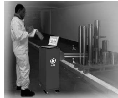
Figure 7: Basic Methodology 3 A trained IAEA inspector operates the LIBS unit on-site. The spectroscopic profile is compared to those in its library to determine the material's make-up and history.
