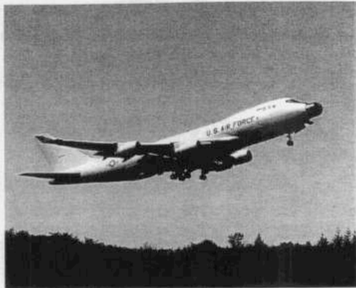
ABL is a modified Boeing 747-400F commercial aircraft with the military designation YAL-1A.
