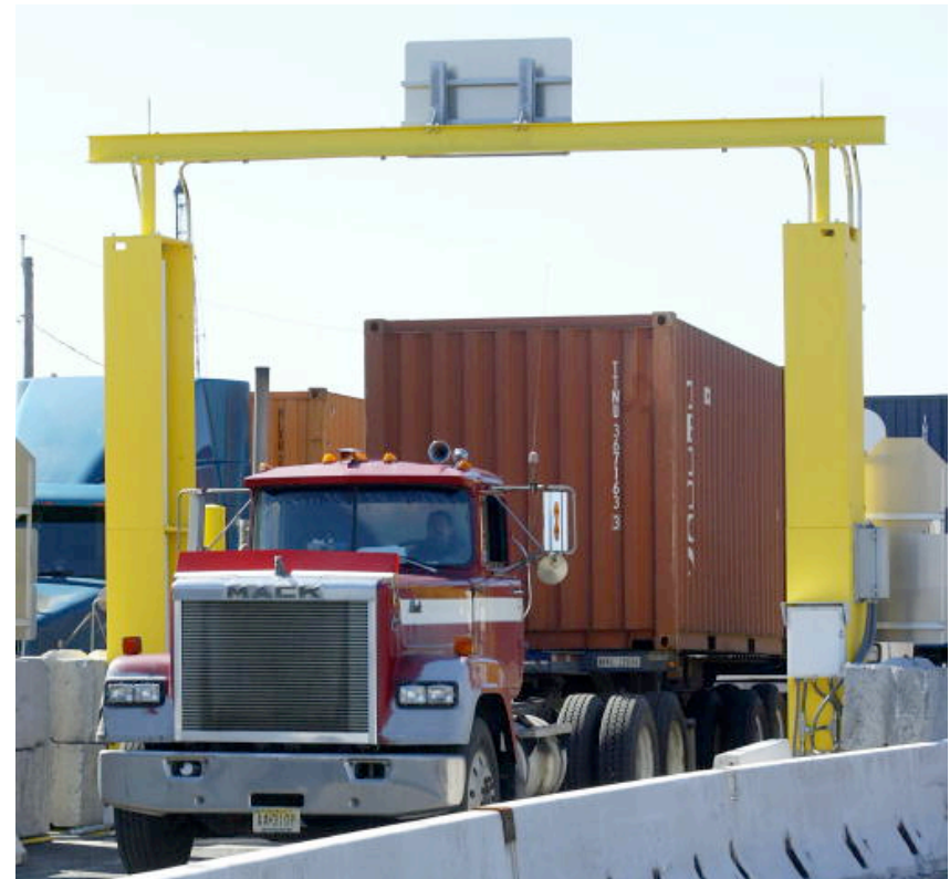
A truck passes through a radiation portal monitor at the port of Newark, New Jersey. http://www.whitehouse.gov/omb/budget/fy2006/dhs.html
