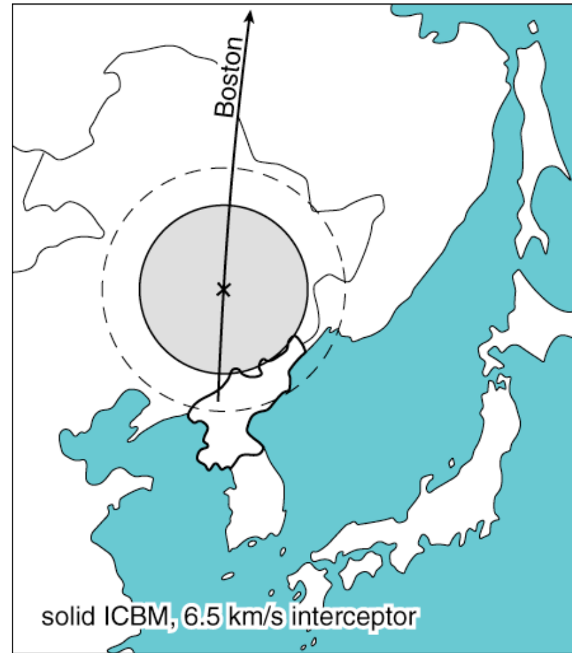
Basing areas for intercepting a solid-propellant ICBM from North Korea to Boston
