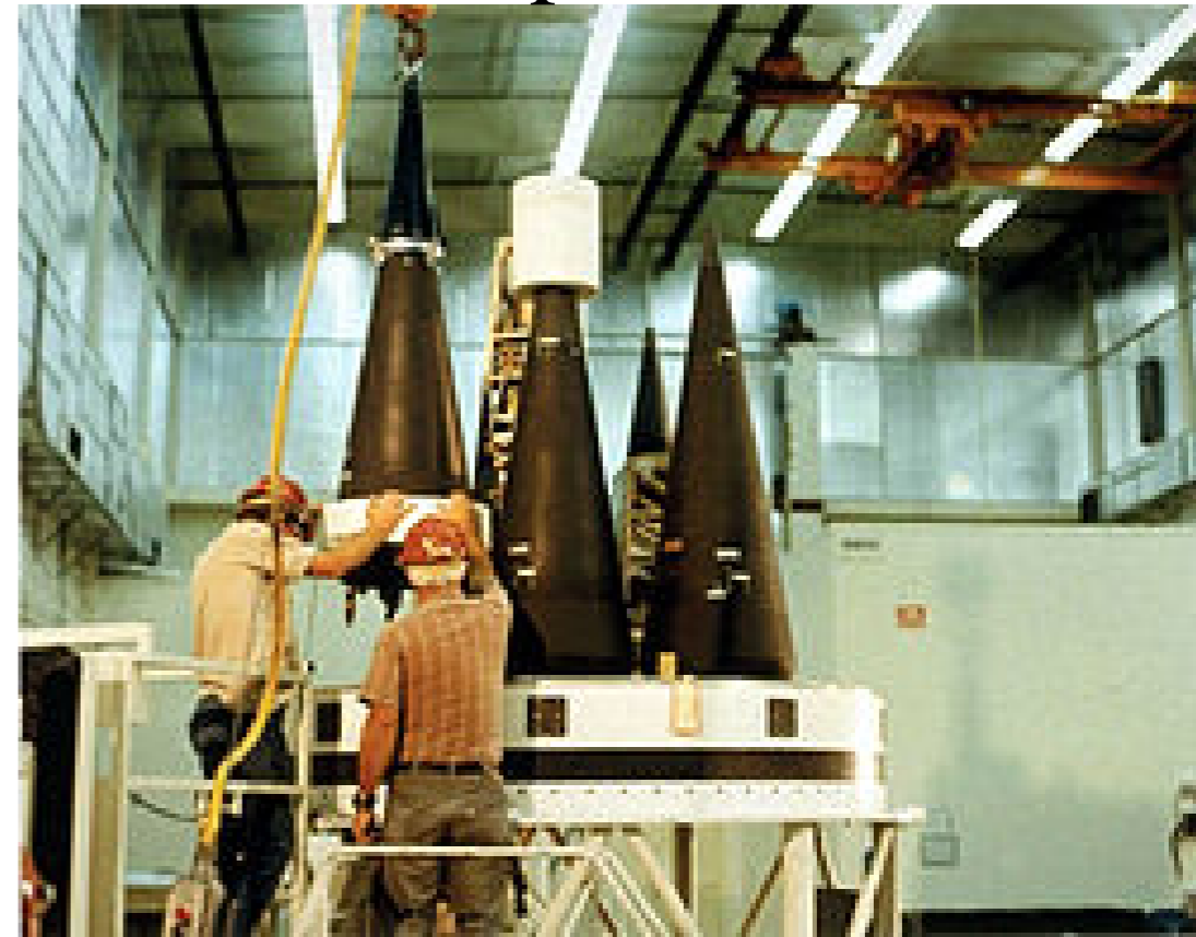
MK21 re-entry vehicles on Peacekeeper MIRV bus
