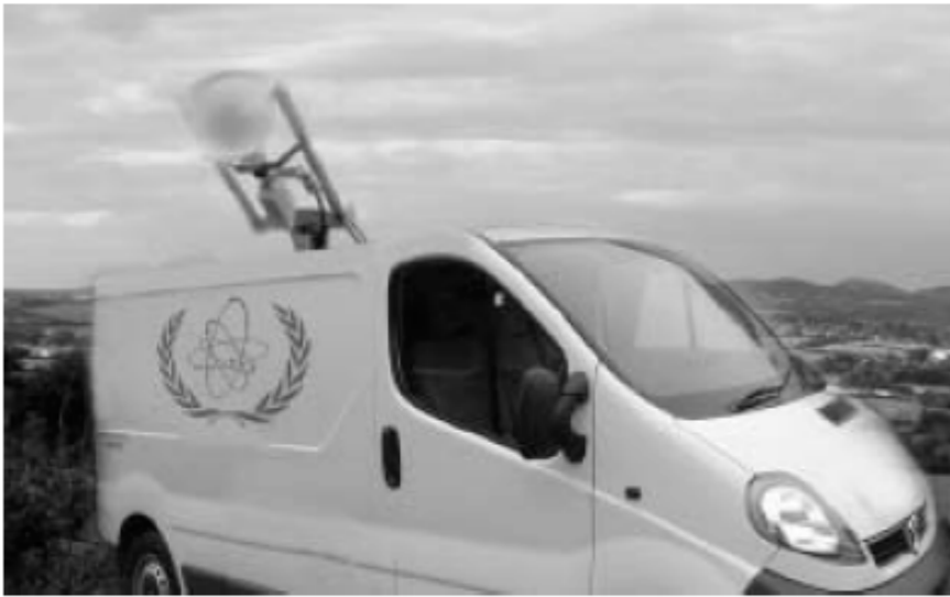
Figure 10: Basic Methodology 1 A mobile on-site laboratory samples and concentrates atmospheric-borne pollutants. Local meteorological conditions and the GPS location are also recorded.
