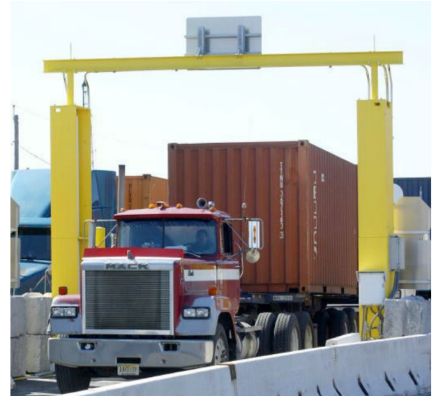
Truck passing through radiation portal monitor at the port of Newark, New Jersey, photo by US Customs and Border Protection
