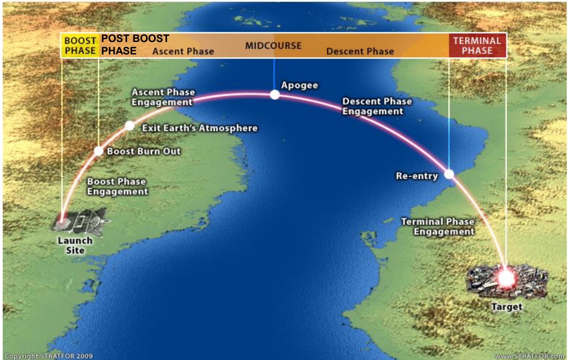
PHASES OF BALLISTIC MISSILE TRAJECTORY
