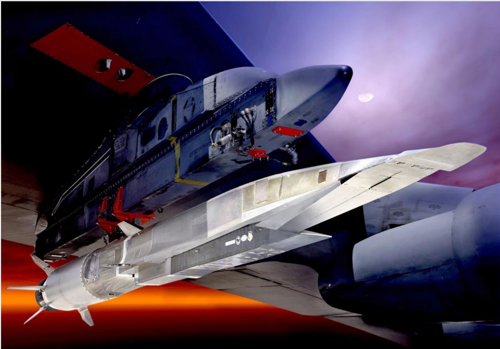
Airbreathing hypersonic missiles would likely be carried by aircraft and employed like conventional cruise missiles. In this design, the US Air Force's experimental X-51 Waverider, shown here under the wing of a B-52 Stratofortress, is set to demonstrate hypersonic flight. Powered by a Pratt & Whitney Rocketdyne SJY61 scramjet engine, it is designed to ride on its own shockwave and accelerate to about Mach 6. Source: US Air Force graphic https://www.af.mil/News/Photos/igphoto/2000360694/
