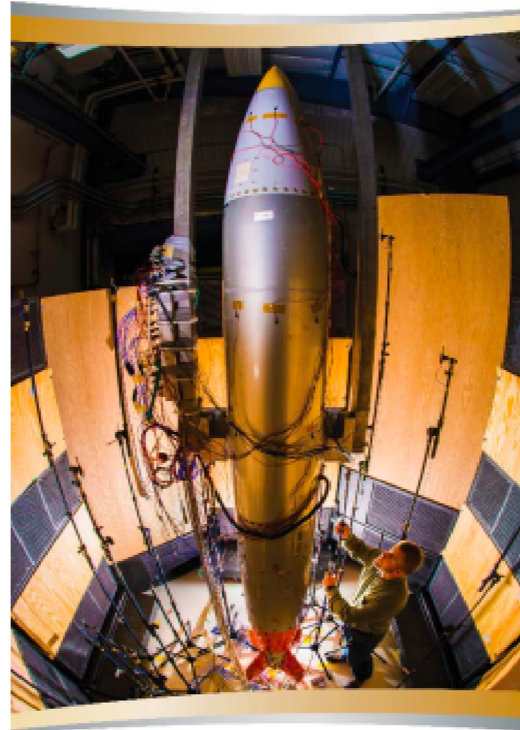
Sandia National Laboratory mechanical engineer adjusts a microphone for an acoustic test on a B-61-12 system.
