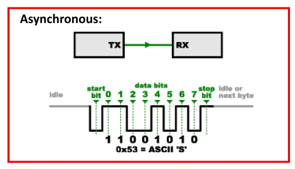
The start bit is always indicated by an idle data line going from 1 to 0, while the stop bit(s) will transition back to the idle state by holding the line at 1.
