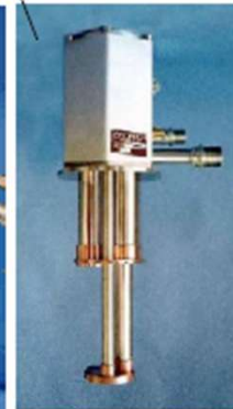
1. Two types of the PTR. (a) A Stirling-type PTR. From left to right it consists of a compressor aftercooler ( X_1 ), a regenerator (reg), a cold heat exchanger ( X_2 ), a pulse tube (tube), a hot heat ( X_3 ), an orifice ( O_1 ), and a buffer. Orifice O_2 connects the hot end of the regenerator and the hot pulse tube. (b) A GM-type PTR. Except for the compressor - rotary valve (r.v.) combination, the ponents of the GM-type PTR are the same as of the Stirling PTR.
