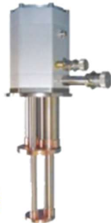
PT 403 First Stage 7W @ 65K Second Stage 0.25W @ 4.2K
