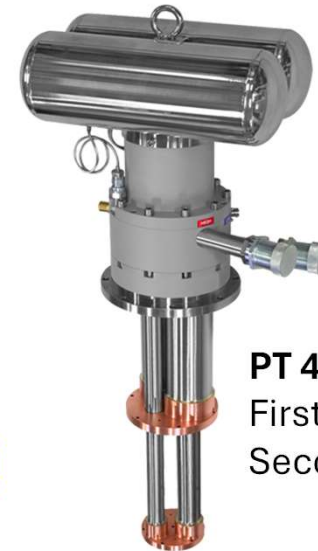
PT 407 First Stage 25W @ 55K Second Stage 0.7W @ 4.2K
