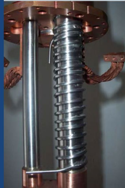
Additional heat exchanger (Uhlig, personal communication)
