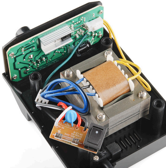
The insides of a soldering iron base
