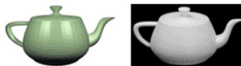
Figure 2. A closed polygonal model of the Utah teapot (left) and the resulting plastic teapot created by rapid prototyping (right).
