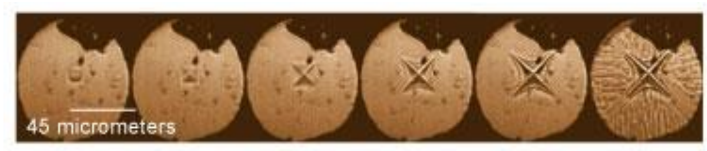
Figure 4. An image sequence from a dDAC experiment shows the growth of a dendritic ice-VI crystal in response to increasing compression. [1]
