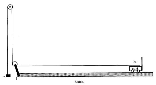
Which is the appropriate relationship between force pulling the cart (F), the mass of the cart (M), the mass of the weight (m), and acceleration of the cart (a)?
