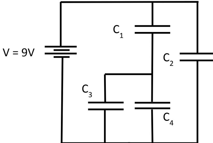
19. What is the equivalent capacitance  $C_{eq}$  of the circuit in terms of  $C=C_1=C_2=C_3=C_4$  ?
