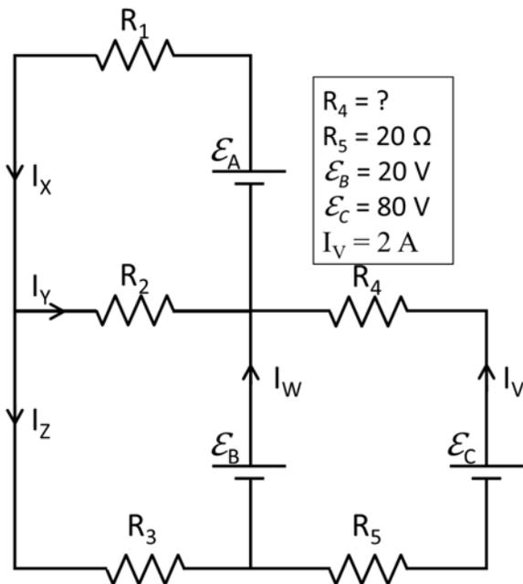
9) What is the resistance of resistor  $R_4$ ?
