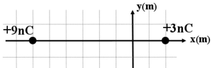
23. Calculate the electric potential at the origin due to the two charges.
