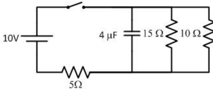
25. What is the current through the 5 Ω resistor immediately after the switch is closed?
