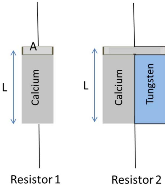
A student decides to build some resistors using rectangular blocks of calcium ( $\rho = 3.36 \times 10^{-8} \Omega \text{ m}$ ) and tungsten ( $\rho = 5.6 \times 10^{-8} \Omega \text{ m}$ ). The dimensions of the blocks are identical with a length  $L = 0.12 \text{ m}$ , and cross section  $A = 2.25 \times 10^{-4} \text{ m}^2$ . Resistor 1 is created from a single block of calcium. Resistor 2 is created by attaching a block of calcium to a block of tungsten as shown in the figure above.
