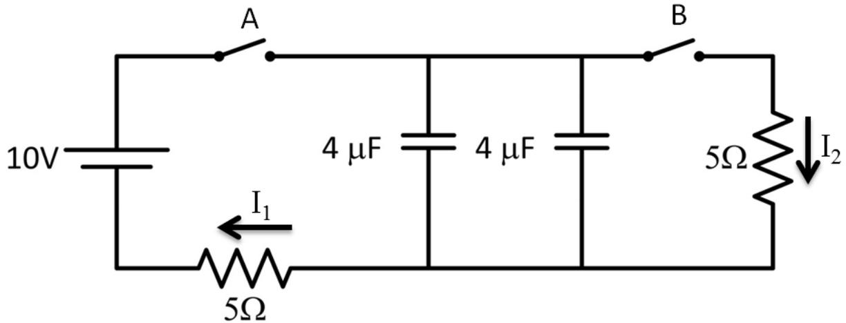
15. Switch B is opened. What is the current  $I_1$  if switch A is left closed for a long time?
