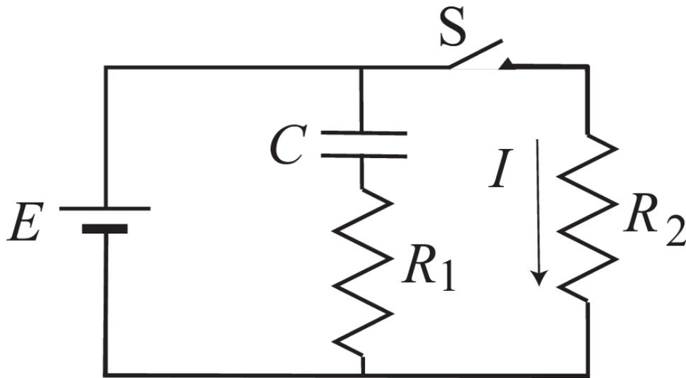
Initially, switch S is open for a long time. After  $t = 0$  switch S is closed. Choose the best figure from below describing the time-dependence of the current  $I$  through  $R_2$ . Do not forget that the battery  $E$  is still connected.
