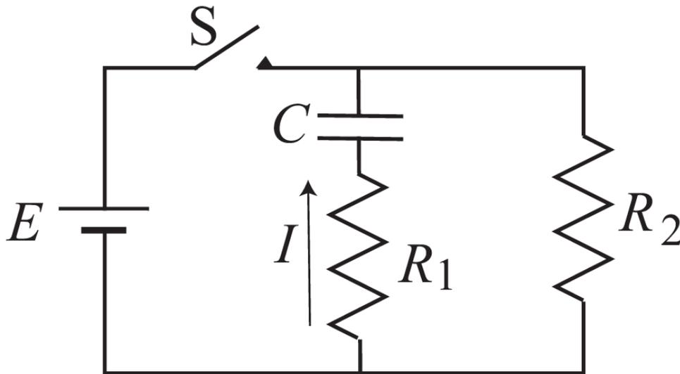
11) Switch  $S$  has been closed for a long time. What is the current  $I$  through  $R_1$  immediately after  $S$  is opened? Pay attention to the direction of the current arrow in the figure.
