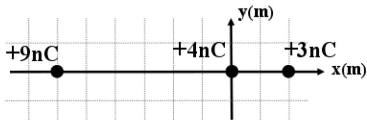
25. What is the speed of the  $4\text{nC}$  charge after it is released and has traveled infinitely far away?
