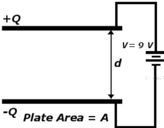
A parallel plate capacitor consists of two metal plates with an area  $A = 542 \text{ mm}^2$  separated by a distance  $d = 0.36 \text{ mm}$ . The capacitor is connected to a 9 volt battery as shown above.
