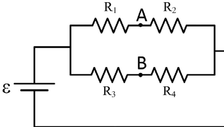
10. How much power is dissipated in this circuit if each resistor has resistance  $R$ ?
