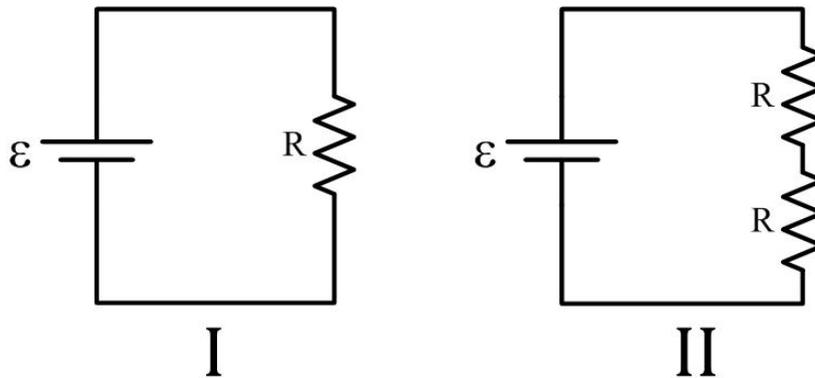
Which of the following statements is true regarding the power  $P_I$  supplied by the battery in circuit I compared with the power  $P_{II}$  supplied by the battery in circuit II?
