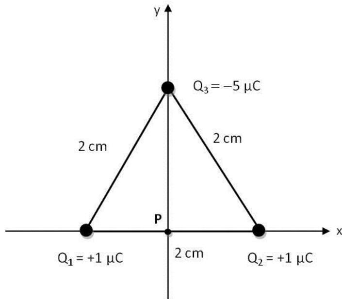
11. How much work  $W$  is required *by you* to assemble the three charges to this configuration?
