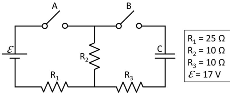
If it takes  $12 \mu\text{s}$  for the charge on the capacitor to drop the 1/2 of its initial value, what is the capacitance of the capacitor C?
