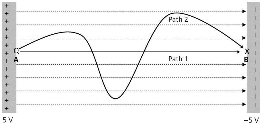
17. Imagine that you move the charge  $Q$  from point **A** to point **B** along the two paths shown. Let  $W_1$  and  $W_2$  be the work done *by the electric field* following Path 1 and Path 2, respectively. What is the relationship between  $W_1$  and  $W_2$ ?
