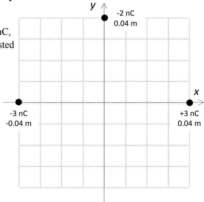
15. What is the electric potential at the position of the  $-2\text{ nC}$  particle, due to the two charges on the  $x$ -axis? The electric potential is defined to be zero at infinity.
