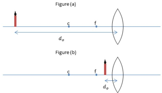
6) The candle is first placed at a distance  $d_o = 14.8 \text{ cm}$  as shown. The image is located at
