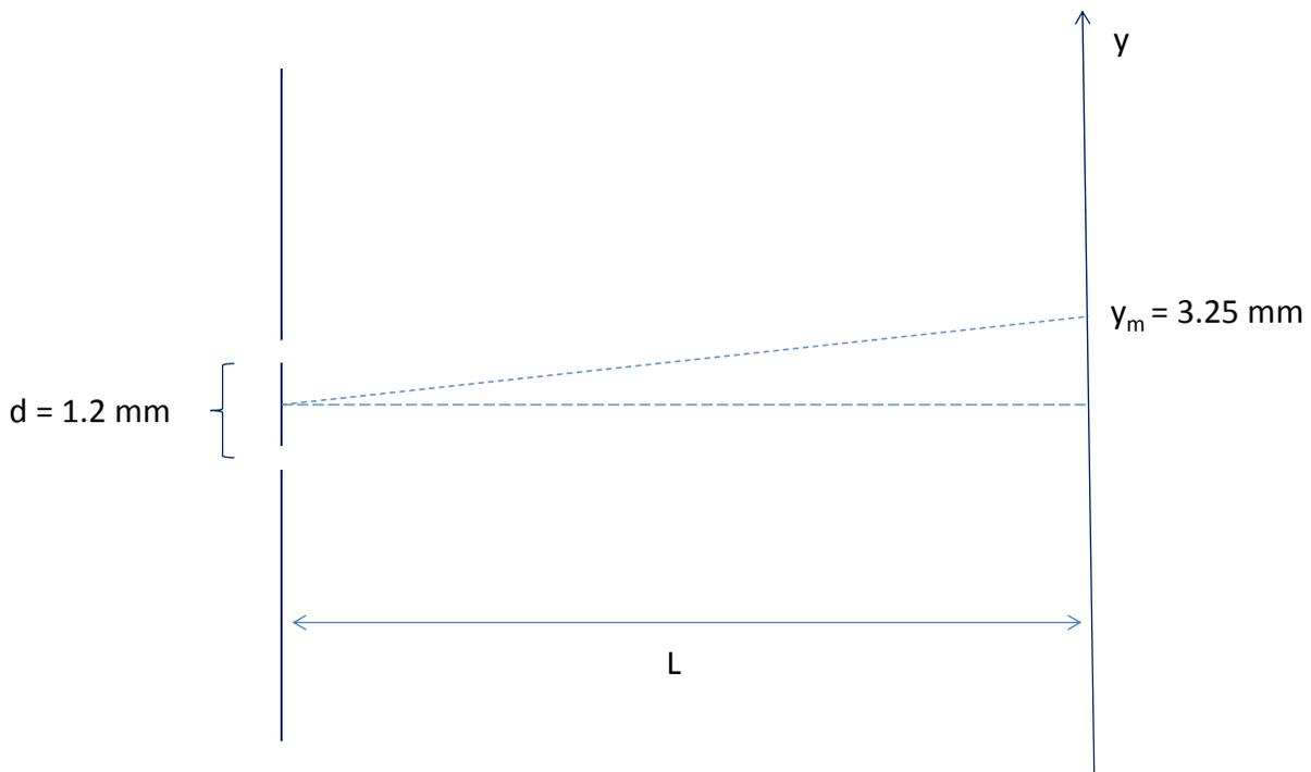
21. A double slit experiment has two slits separated by a distance  $d = 1.2 \text{ mm}$ . Monochromatic (single-wavelength) light is impinging on the two slits with an unknown wavelength. A screen a distance  $L = 2.5 \text{ m}$  away has a third interference maximum ( $m = 3$ ) at  $y = 3.25 \text{ mm}$ . What is the light's wavelength?
