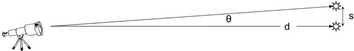
7. The stars are estimated to be separated by  $s = 4.50 \times 10^{11} \text{ m}$ . What minimum diameter of telescope lens is needed to resolve their images?
