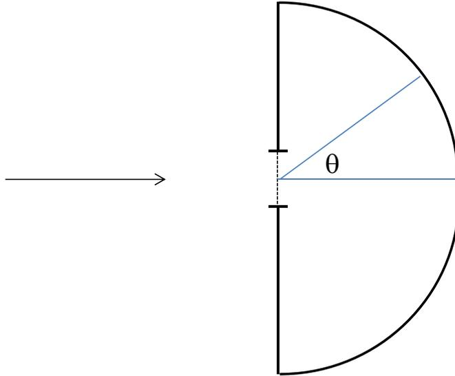
24. A diffraction grating spectrometer has a diffraction grating and a cylindrical screen. The diffraction grating has 8257 slits/cm. Light impinges on the diffraction grating. At which angle  $\theta$  is the 3<sup>rd</sup> order maximum for violet light ( $\lambda = 390$  nm) ?
