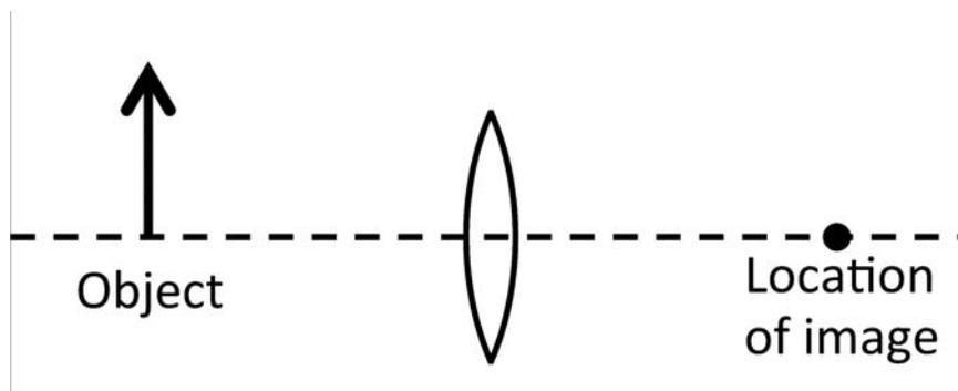
18. Where must one put an object with respect to the convex lens (which has focal length  $f$ ), so that the image is at the same distance from the lens as the object?
