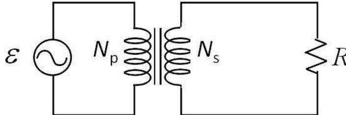
23. Find  $N_s$  for which the maximum induced voltage in the secondary coil is 20 V.
