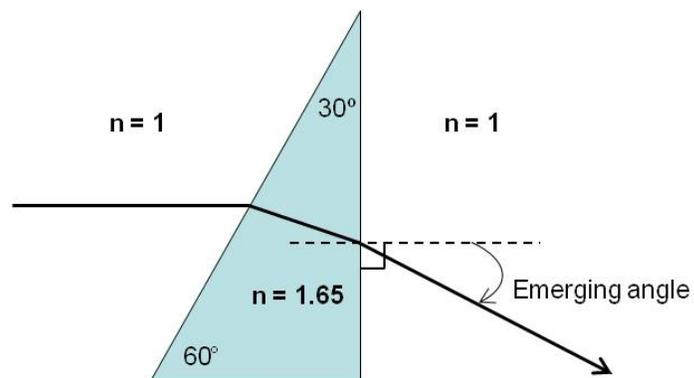
Now assume that the prism is replaced with another one of the same shape but with an index of refraction  $n' = 1.55$ . With respect to the original prism, the emerging angle is
