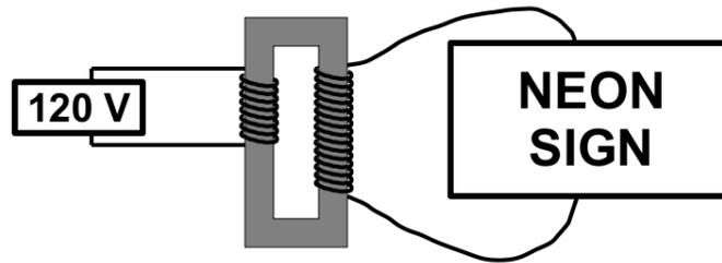
The transformer is designed to have an output voltage of 1200 V when the primary is connected to a 120 V source. How many turns must the secondary winding have if the number of primary turns is 50?
