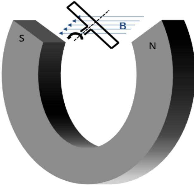
A coil of wire turns between the poles of a permanent magnet as shown in the diagram. The coil has  $N=34$  turns of wire. The magnet produces a constant field of magnitude  $B = 0.119 \text{ T}$ . The coil has a cross-sectional area  $A = 0.0411 \text{ m}^2$ .
