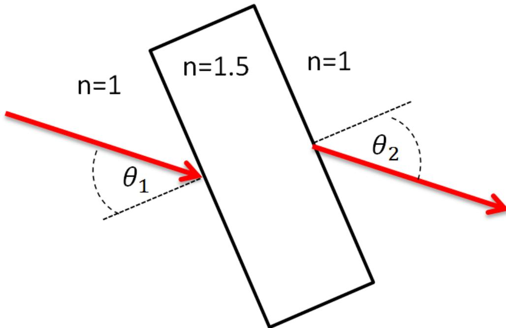
If the angle  $\theta_1=60$  degrees, what is  $\theta_2$ , the angle with respect to the normal on the side of the glass where the beam exits?
