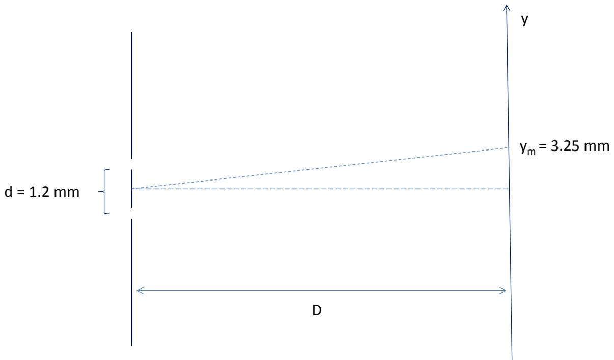
22. The screen is now moved to a new distance  $D$ . A different light source of wavelength  $50 \text{ nm}$  impinges on the two slits. A maximum of order  $m = 2$  now occurs at  $y = 3.25 \text{ mm}$ . What is the new distance  $D$  of the screen from the double slits?
