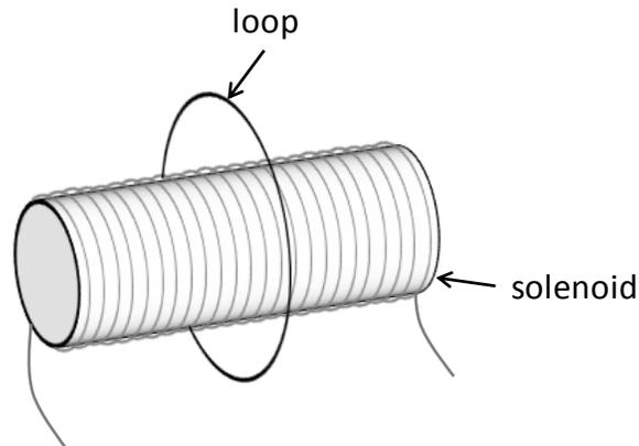
4. Calculate the flux  $\Phi$  through the loop.
