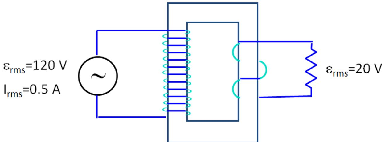
3. What is the rms current on the secondary side of the transformer?
