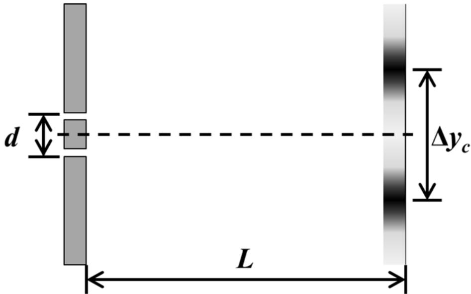
18) What is the distance  $L$  if the width of the central bright spot of the interference pattern is  $\Delta y_c = 1.9 \text{ cm}$ .
