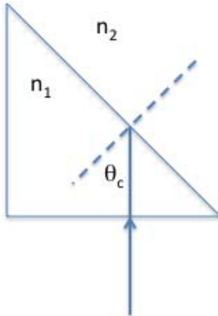
7. What is the index of refraction ( $n_2$ ) of the material in which the prism is immersed?
