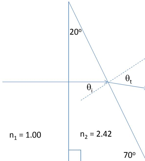
26. A ray of light impinges normally upon a right-angle prism as shown in the diagram above. The prism is made of diamond with an index of refraction  $n_2 = 2.42$ . What is the transmitted angle  $\theta_t$  with respect to the surface normal on the transmission side?
