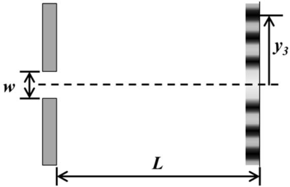
24) At what position  $y_3$  will the third-order ( $m = 3$ ) diffraction minimum be observed?
