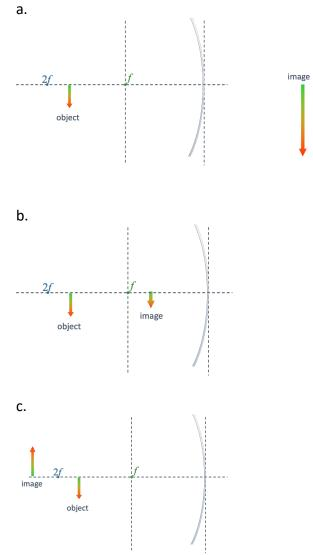
Consider the following optical setup. Light of wavelength 600 nm is incident on a plano-convex lens, made of material whose index of refraction at 600 nm is 1.52. This light is observed to come to a focus 230 cm from the lens (assume thin lens approximation). We now shine in light of wavelength 450 nm, and observe the focus has moved close to the lens by 5 cm.
