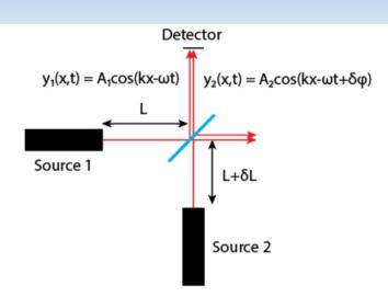
Consider a version of the Michelson interferometer where two independent sources of the same frequency but different amplitude were combined on the beamsplitter, as shown in the figure. With both arms at length L and both sources in phase, the intensity is at a maximum. We then move source 2 by  $\delta L$ .
