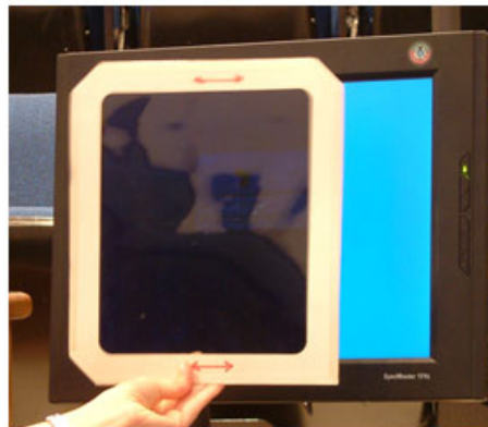
Figure 1: (top) A model of how polarization filters work. If the lines are arranged in opposite ways, the electric field cannot oscillate in either direction, and the light is blocked. (bottom) Light from LCD screens is polarized. If the filter is held one way, you can see the screen, if it's held the other way, it's blocked.
