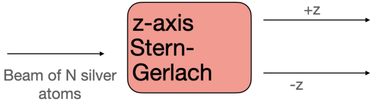
Figure 2: Stern-Gerlach experimental setup. The changing magnetic field separates randomly oriented atoms into two streams.
