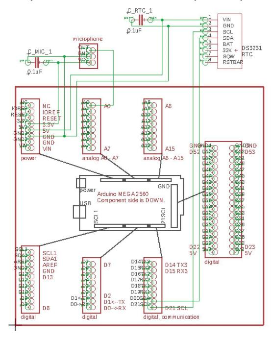
In the circuit, the  $0.1\mu F$  capacitors serve to reduce possible noise injected into the 3.3V and 5V power supply lines. In general it's a good idea to include a capacitor near each device's power/ground inputs.
