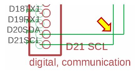
We have two ways of indicating electrical connections. One is to draw lines between various components and pins that are meant to be connected. But this approach can render a complicated circuit impenetrably messy! A better approach is to name various nets, with the understanding that all nets with the same name must be electrically connected by the builder during circuit construction.
