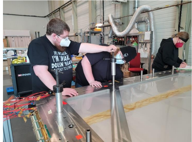
Replacing 20 \mu m W/Au anodes
