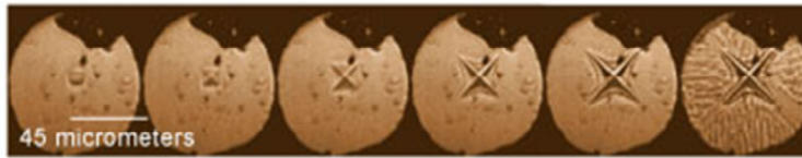
Figure 4. An image sequence from a dDAC experiment shows the growth of a dendritic ice-VI crystal in response to increasing compression. [1]
