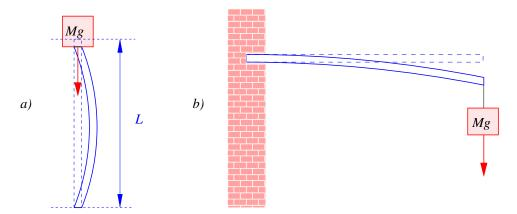
a) Euler's problem: The buckling of a slender column. The rod is used as a column which supports a compressive load Mg directed along the z axis (which is vertical). Show that when the rod buckles slightly (i.e. bends with both ends remaining on the z axis) the total energy, including the gravitational potential energy of the loading mass M, can be approximated by
