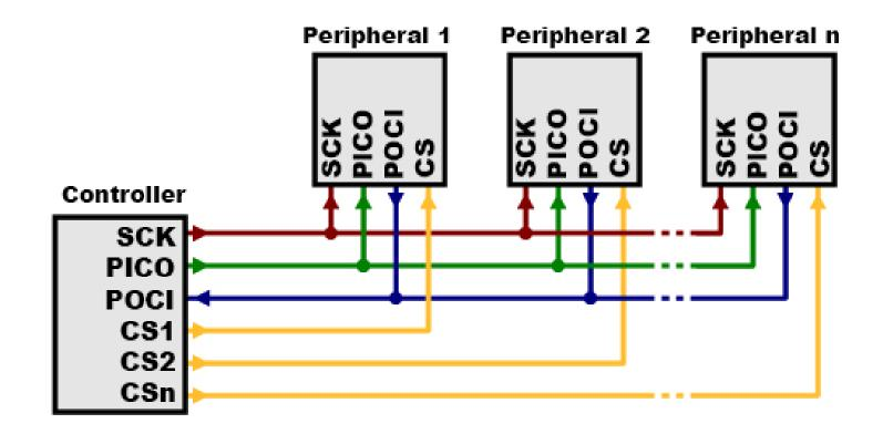
Shared lines for the clock, data in, data out, But requires a separate 'Chip Select' line for each peripheral.
