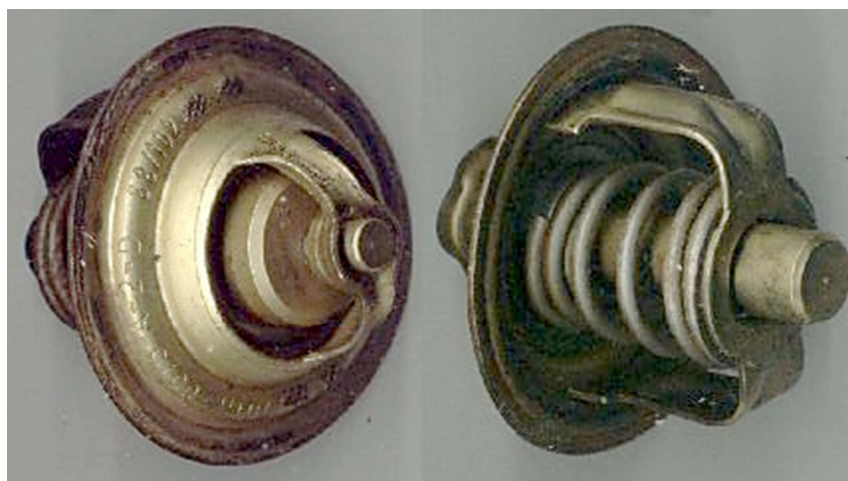
Fig. 1.4: An automobile car engine thermostatic valve. Wax in a hermetic capsule (left photo). Expands with increasing coolant temperature, countering the action of the valve closure spring (right photo) which acts to reduce coolant flow through the radiator when the engine is cold.
