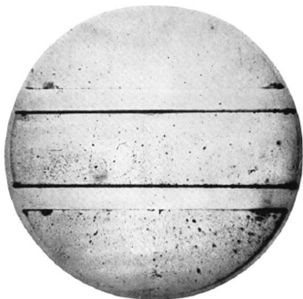
FIG. 4. A positron of about 200 million volts energy ( H\rho = 6.6 \times 10^6 gauss-cm) penetrates the 11 mm lead plate and emerges with about 125 million volts energy ( H\rho = 4.2 \times 10^6 gauss-cm). The assumption that the tracks represent a proton traversing the lead plate is inconsistent with the observed curvatures. The energies would then be, respectively, about 20 million and 8 million volts above and below the lead, energies too low to permit the proton to have a range sufficient to penetrate a plate of lead of 11 mm thickness.
