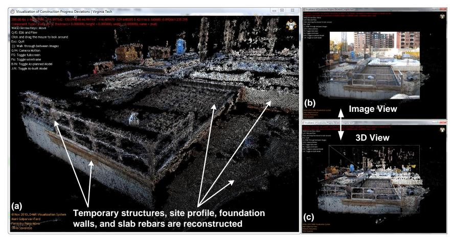
3D reconstruction of a building skeleton elements using <u>12</u> existing images with <u>2Mpixel</u> resolution (Golparvar-Fard 2011)
