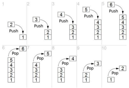
template <class T, class Container = deque<T> > class stack;
