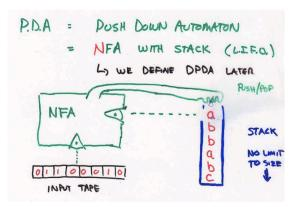
PDAs and CFGs are equivalent: both generate exactly CFLs. PDA is a machine-centric view of CFLs. Helps prove that the intersection of a CFL and a regular language is a CFL.
