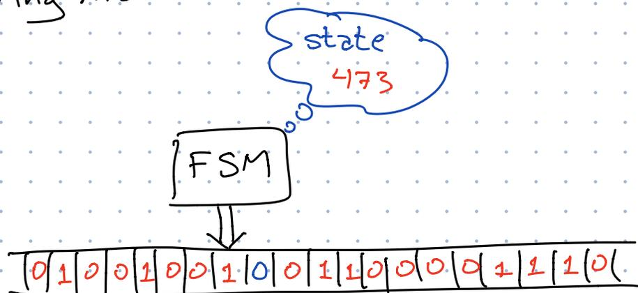
$$\delta: Q \times \Gamma \rightarrow Q \times \Gamma \times \{\Delta, \triangleright\}$$
