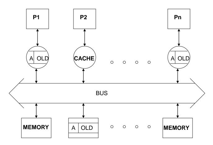
A mechanism needed to propagate a write to other copies
