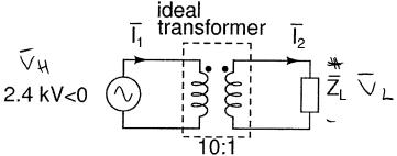
1) Find the load impedance as seen from the high voltage side.
