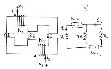
For this problem, you can ignore any resistance in the coil, and any fringing effects in the gaps. The cross sectional area of the core is 1 cm<sup>2</sup>,  $N_1 = 10$ ,  $N_2 = 40$ , g = 1 mm.
