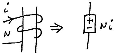
$$W_m = \int_0^\lambda id\hat{\lambda} \quad W_m' = \int_0^i \lambda d\hat{i} \quad W_m + W_m' = \lambda i \quad f^e = \frac{\partial W_m'}{\partial x} = -\frac{\partial W_m}{\partial x} \quad x \rightarrow \theta$$
