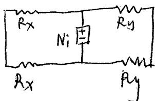
$$\begin{aligned} R_{eq} &= (2R_x) \parallel (2R_y) = \frac{\frac{2x}{\mu_0 AD} \times \frac{2y}{\mu_0 BD}}{\frac{2x}{\mu_0 AD} + \frac{2y}{\mu_0 BD}} \\ &= \frac{\frac{4xy}{\mu_0^2 ab D^2}}{\frac{2xb + 2ya}{\mu_0 ab D}} \\ &= \frac{4xy}{\mu_0 D(2xb + 2ya)} = \frac{2xy}{\mu_0 D(xb + ya)} \end{aligned}$$
