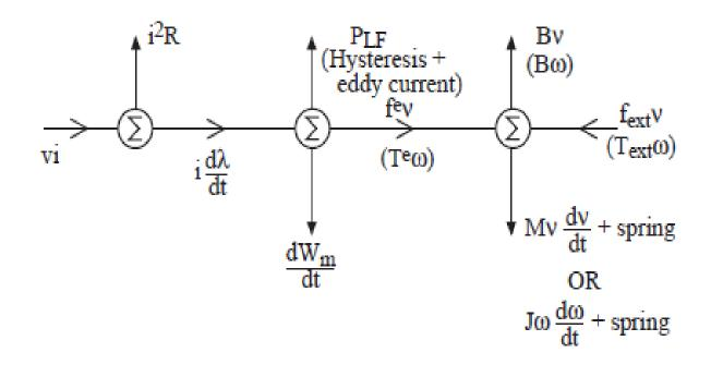
Neglecting the field losses, we get the simple relation for the coupled system (shown dotted)
