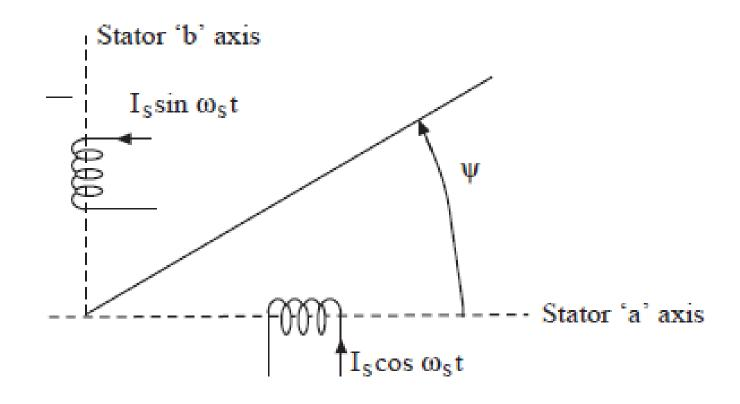
The current in each winding produces a flux density that is maximum along its magnetic axis at some time instant and varies sinusoidally between the positive and negative directions of the axis.
