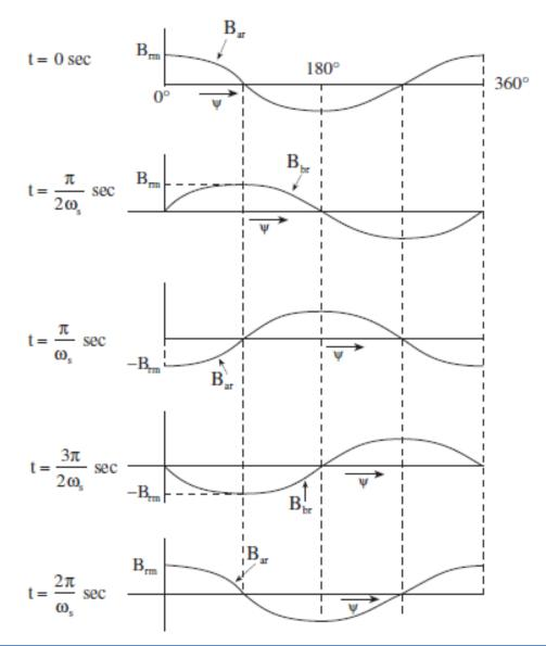
At an arbitrary time instant t, the magnetic field in the air gap at angle  $\psi$  is the sum of  $B_m \sin \omega_s t \sin \psi$  and
