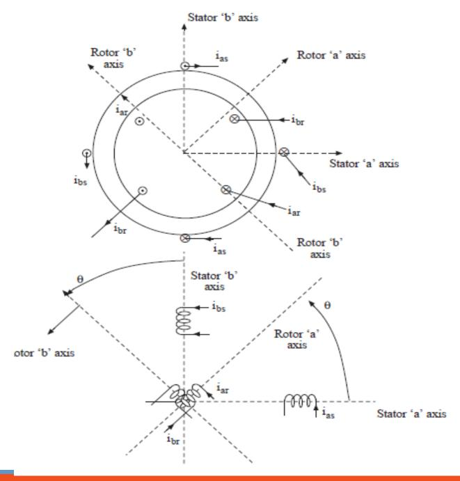
The flux linkage equations can be written by considering each coil coupled with two other coils.
