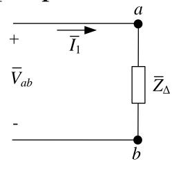
$$\overline{S}_{\Delta,1\varphi} = \overline{V}_{ab}\overline{I}_a^* = \frac{V_{ab}^2}{\overline{Z}_{\Lambda}}$$
