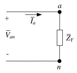
$$\overline{S}_{Y,1\varphi} = \overline{V}_{an} \overline{I}_a^* = \frac{V_{an}^2}{\overline{Z}_Y}$$
