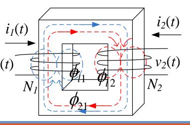
• The polarity markings are assigned such that a positively increasing current in the dotted terminal in one winding induces a positive voltage at the dotted terminal of the other winding
