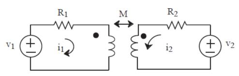
The self induced voltage due to the self inductance is in the direction of the current and is a voltage drop.
